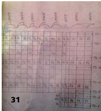
Fig. 31: Assembly maps of Bom Juá's nursery's vaults, which make clear the construction process using prefabricated elements.
