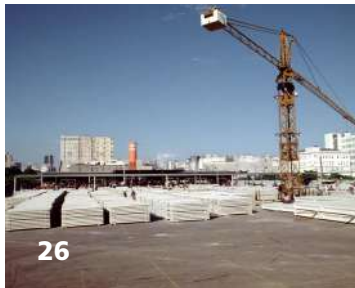
Figs. 24-29: Views of production processes at the School-building Factory, Rio de Janeiro, 1984, Lelé. A more sophisticated sector was built for the 'argamassa armada' elements, as well as curing tanks dedicated to specific pieces, a crane in the storage yard and metallurgy sector for the production of moulds and other metal elements.
