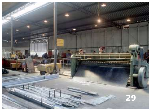
Figs. 24-29: Views of production processes at the School-building Factory, Rio de Janeiro, 1984, Lelé. A more sophisticated sector was built for the 'argamassa armada' elements, as well as curing tanks dedicated to specific pieces, a crane in the storage yard and metallurgy sector for the production of moulds and other metal elements.
