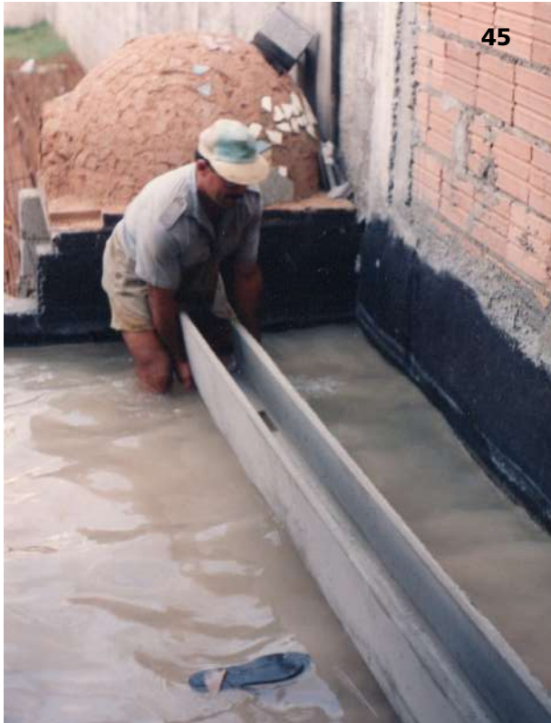
Fig. 44: Curing tanks at the Abadiânia factory, 1983.
