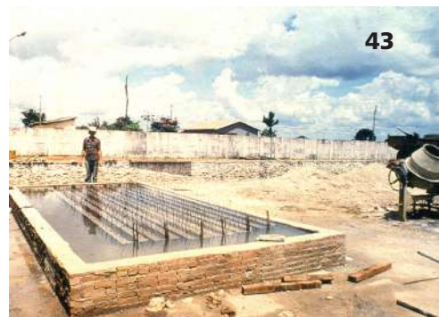
Figs. 40-43: Aspects of the production flow at the Abadiânia factory: framing, mortar production, filling and curing, all within a relatively 'rudimentary' infrastructure, 1983.
